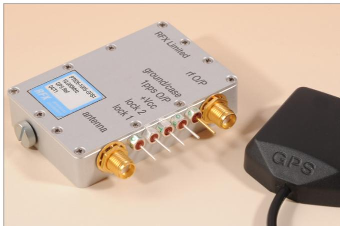
The PT626 - GPS sets a new benchmark for miniature frequency standards. The combination of regulation through the acquisition of GPS data, the storage of control levels, miniature size and integrated OCXO provides a component level module for incorporation into OEM equipment.
